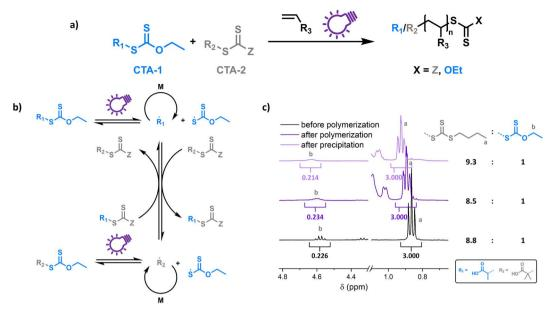
Fig. 1 Schematic representation of XPI-RAFT polymerization (a), and the underlying transfer mechanism from xanthate to CTA-2 (chain transfer between CTAs of equal nature and photo-activation of CTA-2 is not pictured) (b), as well as end group distribution before and after polymerization of a PNAM<sub>10</sub> using a 9:1 mixture of CTA-2 (BABTC) and Xan as monitored by <sup>1</sup>H-NMR spectroscopy (c).
