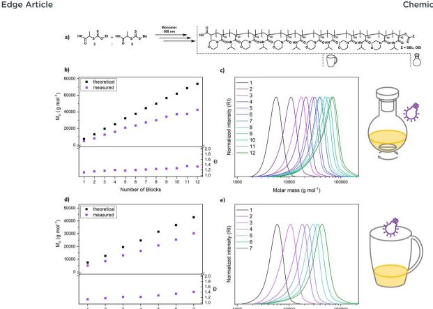
Fig. 6 Synthesis of multiblock copolymers *via* XPI-RAFT polymerization by sequential monomer addition of NAM and NIPAM in an alternating fashion (a). The synthesis was performed in a flask under stirring using a 2 W lamp (b and c), as well as in a coffee mug without stirring or degassing, and under open-to-air conditions using a 4 W lamp (d and e).
