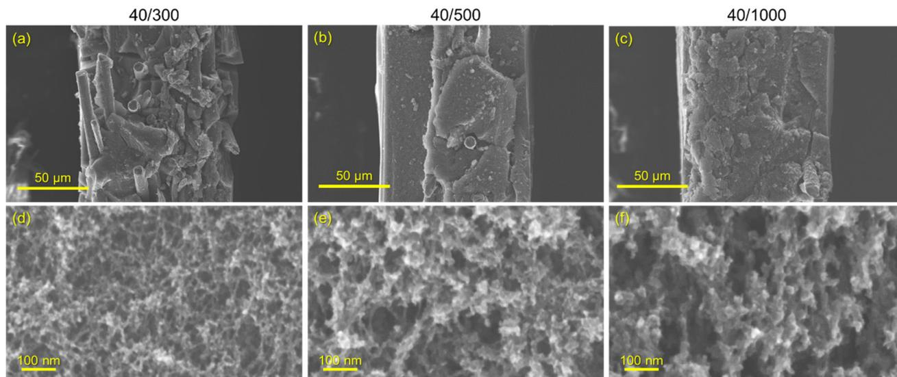
**Fig. 1** Scanning electron micrographs of 1-ply CNFP cross-sections for CNFP-40/300 (a), CNFP-40/500 (b), and CNFP-40/1000 (c), and their respective magnified images (d–f). In (a–c), the carbon nanofoam appears as a solid filling the gaps in the carbon fiber paper, and the pores are only visible at much higher magnifications (d–f).
