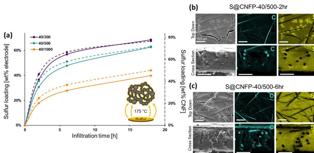
**Fig. 3** (a) Mass uptake by CNFPs upon vapor infiltration of  $\text{S}_8$  as a function of time: solid line represents the measured mass uptake in the CNFP, and the dotted line shows the mass of  $\text{S}_8$  uptake relative to the carbon nanofoam component of the CNFP. Scanning electron microscopy and cross-sectional EDS analysis of C and S for (b) 2 h and (c) 6 h infiltrations.
