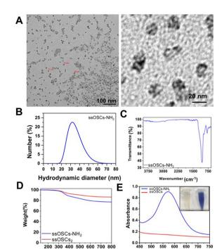
Fig. 1 Characterization of the breakable ssOSCs-NH<sub>2</sub>. (A) Transmission electron microscopy images of the ssOSCs functionalized with NH<sub>2</sub> groups. (B) DLS analysis, (C) FTIR spectrum, (D) TGA of ssOSCs-NH2 compared to ssOSCs. (E) Kaiser test for determining primary amines with the maximum absorption peak at 570 nm.
