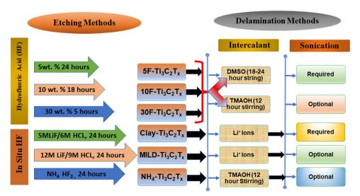
Fig. 2 Schematic diagram of the synthesis route of Ti<sub>3</sub>C<sub>2</sub>T<sub>x</sub> MXene. Reproduced with permission from ref. 58 Copyright 2020. MDPI (open Access).
