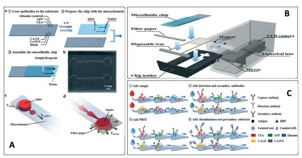
Fig. 3 (A) Basic design & assembly of the chip (a). Microfluidic chip (b). Inlet & outlet of the chip showing the capillary action (c) and (d). (B) Schematic of the POC chip for cancer detection. (C) Detection process of the assay for different cancer biomarkers. Reproduced from ref. 42 with permission from the Royal Society of Chemistry.
