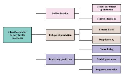
Classification of objectives and the corresponding methodologies for battery health prognostics.
