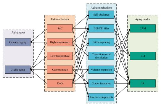
Influencing factors on aging side reactions and the corresponding aging types
