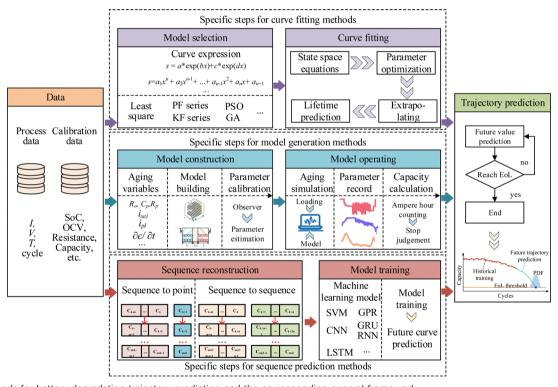
Fig. 12 Methods for battery degradation trajectory prediction and the corresponding general framework
