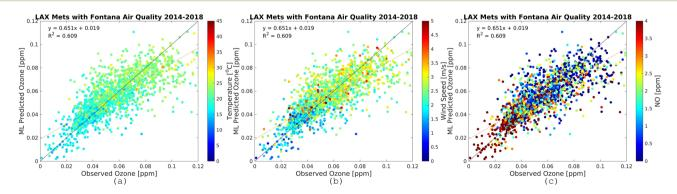
Fig. 7 Observational O<sub>3</sub> (x-axis) and RFR predictions (y-axis) for Fontana air quality and meteorology from the LAX international airport monitoring station. The plots are for the most recent five-year increment from 2014-2018. The color bars show temperature (a), wind speed (b), and NO (c). Plots for other periods are provided in the ESI.†
