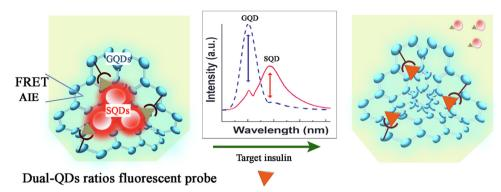
Fig. 6 The sensing mechanism of the dual-QDs ratios fluorescent probe. Adapted with permission from ref. 93. Copyright 2021 Elsevier B.V.
