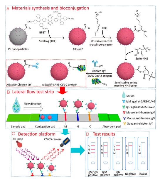
Fig. 5 Diagram of AIE nanoparticles-labelled lateral flow immunoassay for detection of virus. (A) Synthesis of AIE<sub>810</sub>NPs and conjugation path of SARS-CoV-2 antigen and chicken IgY. (B) Schematic of test strip for the detection of IgM and IgG against SARS-CoV-2. (C) Schematic of the portable reader. (D) Interpretation of different test results. Adapted with permission from ref. 82. Copyright 2021 American Chemical Society.
