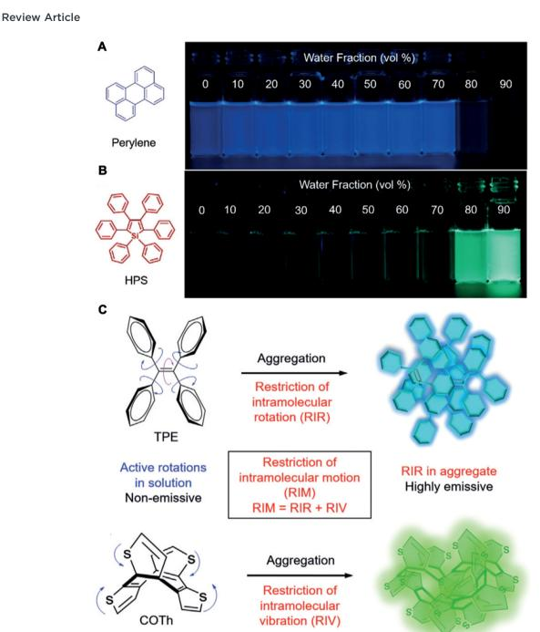
Fig. 1 Molecular mechanism of AlEgens. (A) Molecular structures and photographs of a typical ACQ molecule (perylene) and (B) an AIE molecule (hexaphenylsilole, HPS). (C) Schematic of the AIE mechanism of the restriction of intramolecular motion (RIM). Adapted with permission from ref. 14. Copyright 2020 Wiley-VCH Verlag GmbH & Co. KGaA, Weinheim.
