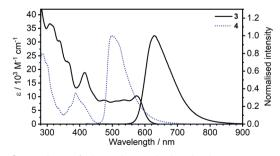
Fig. 1 Comparison of absorption and photoluminescence spectra of complexes **3** and **4** in toluene,  $c = 10^{-5}$  M for absorption and c = $5 \times 10^{-7}$  M for emission spectra.
