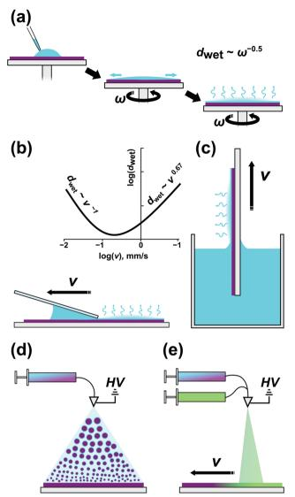
Fig. 4 BCP film casting methods. (a) Spin-coating. (b) Blade-coating. (c) Dip-coating. (d) Electrospray deposition of a polymer film with a homogeneous composition and (e) with a lateral composition gradient.
