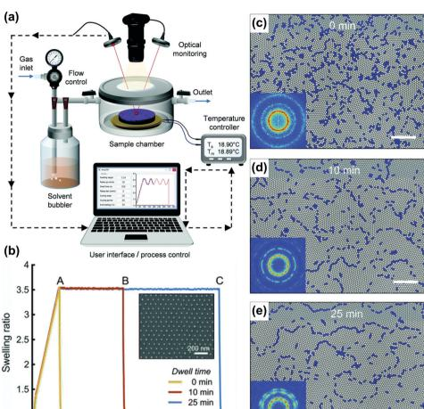
Fig. 8 Automated solvent vapor annealing. (a) Schematic of an advanced SVA setup with closed-loop SR control. (b) Annealing pathways of cylinderforming PS-b-P2VP 258 kg mol<sup>-1</sup> thin films in THF vapor and corresponding morphologies after 0, 10, and 25 min (c-e). Adapted from Soft Matter, 15, 7909.<sup>176</sup> With permission from The Royal Society of Chemistry.
