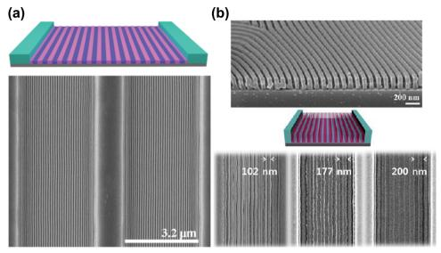
Fig. 11 Solvent vapor-assisted graphoepitaxial ordering of high MW PS-b-PMMA lamellar patterns. SEM images of films in trench confinement. (a) 3.2 μm wide trench; (b) cross-section view and top-down images of 1.5 μm wide trench. Reprinted with permission from Macromolecules, 49, 1722, 88 and ACS Nano, 7, 1952. 159 Copyright 2016, 2013 American Chemical Society
