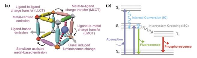
Fig. 6 (a) Schematic diagram of various origins of luminescence in LMOFs. (b) Illustration of photon emission in ligand-centred luminescence. Adopted from ref. 151.
