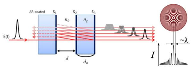
Fig. 8 Illustration of the working principle of a Fabry-Perot interferometer and a typical Fabry-Perot interference pattern.
