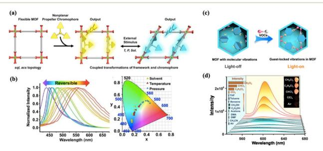
Fig. 7 (a) Illustration of the organic chromophore 3-TPPA grafted in the dynamic coordination space of a flexible MOF. (b) Wide-range emission colour tuning of a 3-TPPA grafted MOF-105 material.  $^{107}$  (c) Illustration of the guest-induced luminescence enhancement mechanism in the presence of VOCs. (d) Emission spectra of  $[Cu_4I_4(Py_3P)_2]_n$  after incubation for 30 min in various solvent vapours.  $^{108}$
