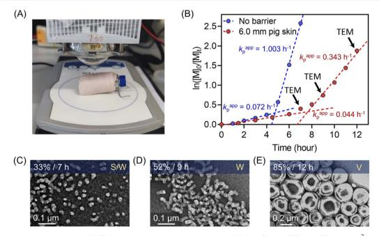
Fig. 7 (A) Experimental setup of photo-RAFT dispersion polymerization under the NIR light ( $\lambda_{max}=730$  nm; 60 mW cm<sup>-2</sup>) irradiation passing through 6.0 mm pig skin. (B) Comparison of dispersion photo polymerization kinetics between without barrier and through 6.0 mm pig skin. (C–E) Evolution of morphologies of polymeric nanoparticles synthesized through 6.0 mm pig skin indicated by corresponding TEM images at different time points (t=7, 9, and 12 hours).
