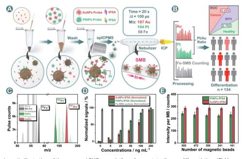
Fig. 1 (A) and (B) schematic illustration of the proposed SMB nanoplatform for prostate disease differentiation. (C) Mass scanning of magnetic beads, AuNPs, and PtNPs. (D) Dual-biomarker evaluation using the SMB nanoplatform with the same number of magnetic beads. (E) Stable data processing of the SMB nanoplatform with varied numbers of magnetic beads.
