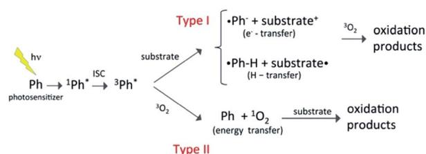
Fig. 1 Schematic representation of different types of photosensitization process,<sup>3,4</sup> where the photosensitizer excited to a triplet state reacts with a substrate by electron or hydrogen transfer, or transfers energy to triplet molecular oxygen. In the latter case, the oxygen molecule is excited to the singlet state that then reacts with the substrate.
