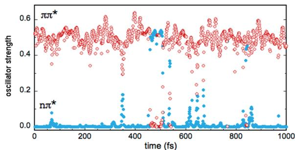
Fig. 7 Fluctuations of the oscillator strengths for  $S_0 \rightarrow S_1$  (blue plain circles) and  $S_0 \rightarrow S_2$  (red open circles) electronic transitions over one picosecond of the QM/MM MD simulation of IC in bulk water. The values for transitions with mainly ( $n\pi^*$ ) or ( $\pi\pi^*$ ) character are indicated.
