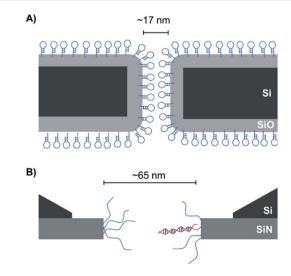
Fig. 11 Solid-state nanopores modified using 1,4-phenylene diisothiocyanate as a cross-linking agent to attach amino-terminated (A) DNA hairpins<sup>56</sup> and (B) single-stranded DNA.<sup>57</sup> The passage of complementary strands through such pores was slowed, resulting in prolonged ion current drops.
