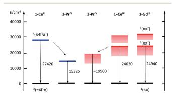
Fig. 6 Partial electronic diagram for 1-Ce,  $3\text{-Pr}^{\text{MecN}}$ , and 1-Gd. Calculated levels in blue, experimental 0-phonon levels in red or rose when estimated from the onset of the emission band. Energies of the transitions in cm $^{-1}$ .
