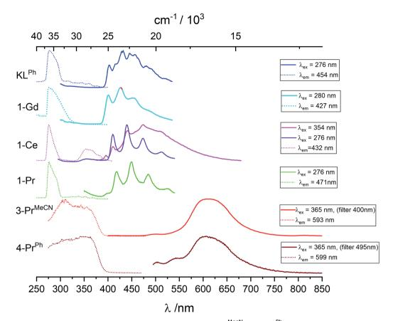
Fig. 5 Excitation and emission spectra of KOSiPh<sub>3</sub>, 1-Ln (Ln = Gd, Ce, Pr),  $3-Pr^{MecN}$  and  $4-Pr^{Ph}$  in 5 mM toluene solution at 77 K. Spectra are normalized and their intensities cannot be directly compared.
