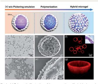
**Fig. 1** (a) Schematic illustration of the preparation of hybrid microgels. (b) Optical micrograph of the w/o Pickering emulsion template. (c-e) SEM images of the dried hybrid microgels. (f) CLSM image of the hybrid microgels and the inset shows the hollow structure of the microgel. (g) 3D reconstruction of the hybrid microgel dispersed in water *via* a z-stack of CLSM images. The red color indicates rhodamine B-labelled PNIPAM.
