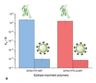
Fig. 5 (A) Binding isotherms of SARS-CoV-2 VLP and RBD formulated in PBST to GFNCYFPLQ-imprinted polyscopoletin spots as revealed by SPRi. (B) Comparison of the  $K_D$  values for the interaction of VLP and RBD with hepta-and nonapeptide imprinted polymer nanofilms. The  $\mathcal{K}_{\mathsf{D}}$  values for the VLPs should be considered estimates given the limitation of the SPR technique to assess subpicomolar  $K_D$  values.
