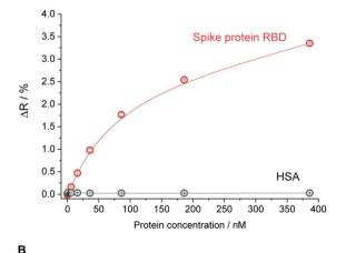
Fig. 3 The selectivity of the epitope-imprinted polymer microarray. (A) The differential SPR images of the MIP chip for the layout shown in Fig. 2A exposed to RBD and HSA. (B) Binding isotherms of RBD and HSA to the nonapeptide GFNCYFPLQ-imprinted polyscopoletin spots recorded in PBST.
