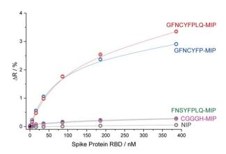
Fig. 2 (A) The SPR image and microspotting layout of the epitope-imprinted polymer microarray. Each peptide concentration was spotted in triplicates. The diameter of the spots is  $\it ca. 500~\mu m$  with 420  $\it \mu m$  spacing. (B) RBD binding to the different peptide-imprinted polyscopoletin spots.
