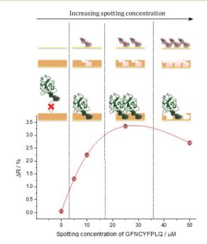
Fig. 1 The effect of the microspotted GFNCYFPLQ peptide concentration on the subsequent binding of RBD at its saturation concentration (385 nM) to the respective epitope-imprinted spots in phosphate buffer saline with 0.05% Tween 20 (PBST). The reflectivity change  $(\Delta R)$  is indicative of the amount of bound RBD, i.e. the binding capacity of the respective MIP spots.
