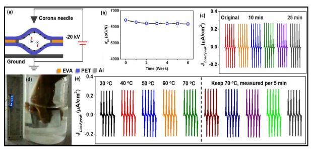
Fig. 23 Verification of PET/EVA PENG sample via (a) corona poling, and (b) d<sub>33</sub> coefficient consistency over a six-week period; (c) stability of the generator under high moisture conditions; (d) illumination of six LEDs by pressing the device underwater; and (e) current output of the flexible PENG at high temperature (70 °C); reproduced with permission from ref. 309. Copyright 2017, Elsevier publication.
