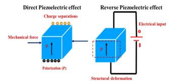
Fig. 1 Direct and reverse piezoelectric effect.
