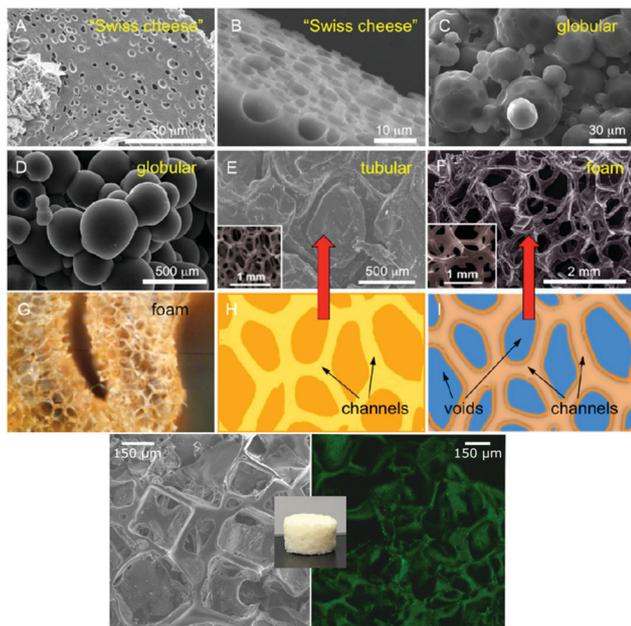
**Fig. 1** Top: SEM images of the internal porosity of: smectic LCE- $\gamma$  (A) before, (B) and after 16 weeks of biodegradation in PBS, (C and D) of globular, porous microstructure of nematic LCE (E) LCEPP, (F) LCEPP, (G) optical image of LCEFP + SP. Scheme of type de foams used to fabricate: (H) LCEPP, and (I) LCEFP + SP. Reprinted (adapted) with permission from ACS<sup>(C)</sup> Symposium series ref. 4. Copyright 2017 American Chemical Society. Bottom: Adapted from ref. 65 RSC Soft Matter.
