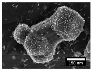
Fig. 4 Micrograph showing zinc electrodeposited after 5 s near one of the edges of the electrode using a current density of 150 A  $m^{-2}$ . The hexagonal nanoflakes are visible as merging with its surface.
