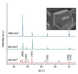
Fig. 3 XRD diffractograms of zinc deposited at current densities of 150 A m $^{-2}$ , 500 A m $^{-2}$  and 1000 A m $^{-2}$ . The peaks corresponding to the titanium phase (JCPDS-ICDD, 44-1294) are labelled with a black square ( $\blacksquare$ ). The hexagonal prism analogous to the zinc crystal in Fig. 1f illustrates the corresponding directions of the crystal planes (002) and (100).
