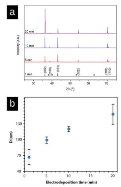
Fig. 5 (a) XRD patterns of zinc-deposition on the surface of the Ti substrate at a current density of 1000 A m<sup>-2</sup> depending on electrodeposition times. 1 min (black); 6 min (red); 10 min (blue); and 20 min (pink). The peaks corresponding to titanium are labeled with a black square (1). (b) Crystallite size (D) as estimated with the Scherrer equation measured for four different electrodeposition times at a current density of 1000 A m<sup>-2</sup>.
