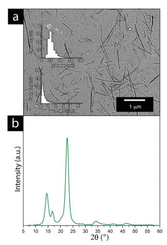
**Fig. 6** (a) TEM micrographs of the bacterial cellulose obtained after acid hydrolysis, including histograms showing the length and thickness distributions of the bacterial cellulose. (b) XRD diffractogram of the bacterial CNF obtained after acid hydrolysis.
