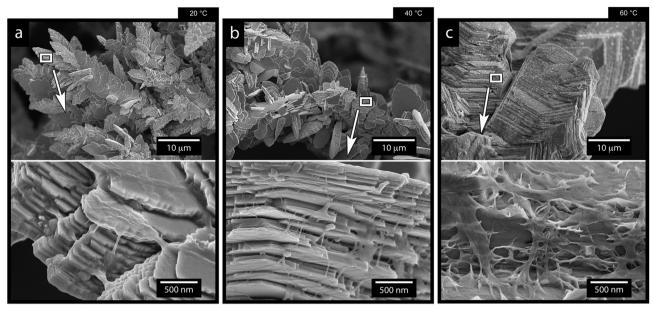
Fig. 9 SEM micrographs of the zinc electrodeposited Ti-electrodes after 7 min of electrodeposition at a current density of 1000 A  $m^{-2}$ , a CNF concentration of 0.5 g  $L^{-1}$ , and temperatures of 20 °C (a), 40 °C (b) and 60 °C (c). A figure serving as the reference, describing the electrodeposition in the absence of cellulose at different temperatures are provided in in Fig. S15 (ESI†).
