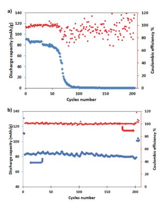
Fig. 7 Long term cycling (blue) and coulombic efficiency (red) of (a) NMO and (b) NMCO for 200 cycles at C/2 (after a pre-conditioning for 5 cycles
