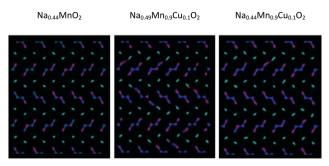
Fig. 10 Comparison among the Na<sup>+</sup> ion trajectories at 700 K for a given occupation of the Na1 crystallographic sites (60%) as the composition changes: view along the c axis.
