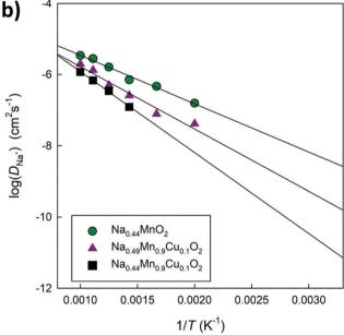
Fig. 12 Arrhenius plot of Na<sup>+</sup> diffusion coefficients (D) for (a) two different models having the same composition (Na<sub>0.44</sub>MnO<sub>2</sub>) and characterized by a different distribution of Na+ ions between 1D and 2D channels; and (b) three different models having the same occupation of the Na1 site (60%) but different composition.
