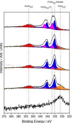
Fig. 6 XPS Au(4f)/Pt(4f) and Pd(3d)/Au(4d) spectra for as-prepared 0.66%AuPdPt/TS-1 catalysts, prepared by sol-immobilisation (PVA: metal = 1.2). (a) 0.33%Au-0.33%Pd/TS-1, (b) 0.275%Au-0.275%Pd-0.11%Pt/TS-1, (c) 0.22%Au-0.22%Pd-0.22%Pt/TS-1 (d) 0.11%Au-0.11%Pd-0.44%Pt/TS-1 and (e) 0.66%Pt/TS-1. Note: all catalysts were exposed to an oxidative heat treatment prior to use (static air, 400 °C, 3 h).
