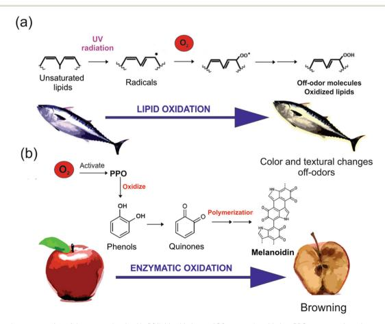
Fig. 5 Schematic representation of the process involved in (a) lipid oxidation and (b) enzymatic oxidation. PPO corresponds to the enzyme polyphenol oxidase.
