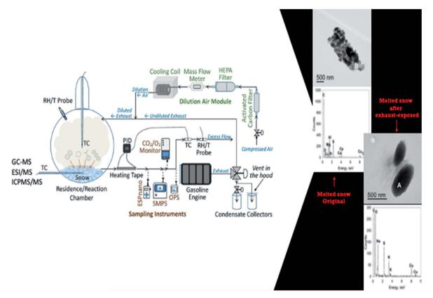
Fig. 6 At LHS, a simplified schematic of snow chamber-exhaust facility is shown. 16 At RHS, high-resolution transmission electron microscopy (HR-TEM) with energy dispersive spectroscopy (EDS) of duplicate melted snow samples in a site before and after exhaust exposure, are illustrated. An increase of particles in snow upon gasoline exposure was also observed
