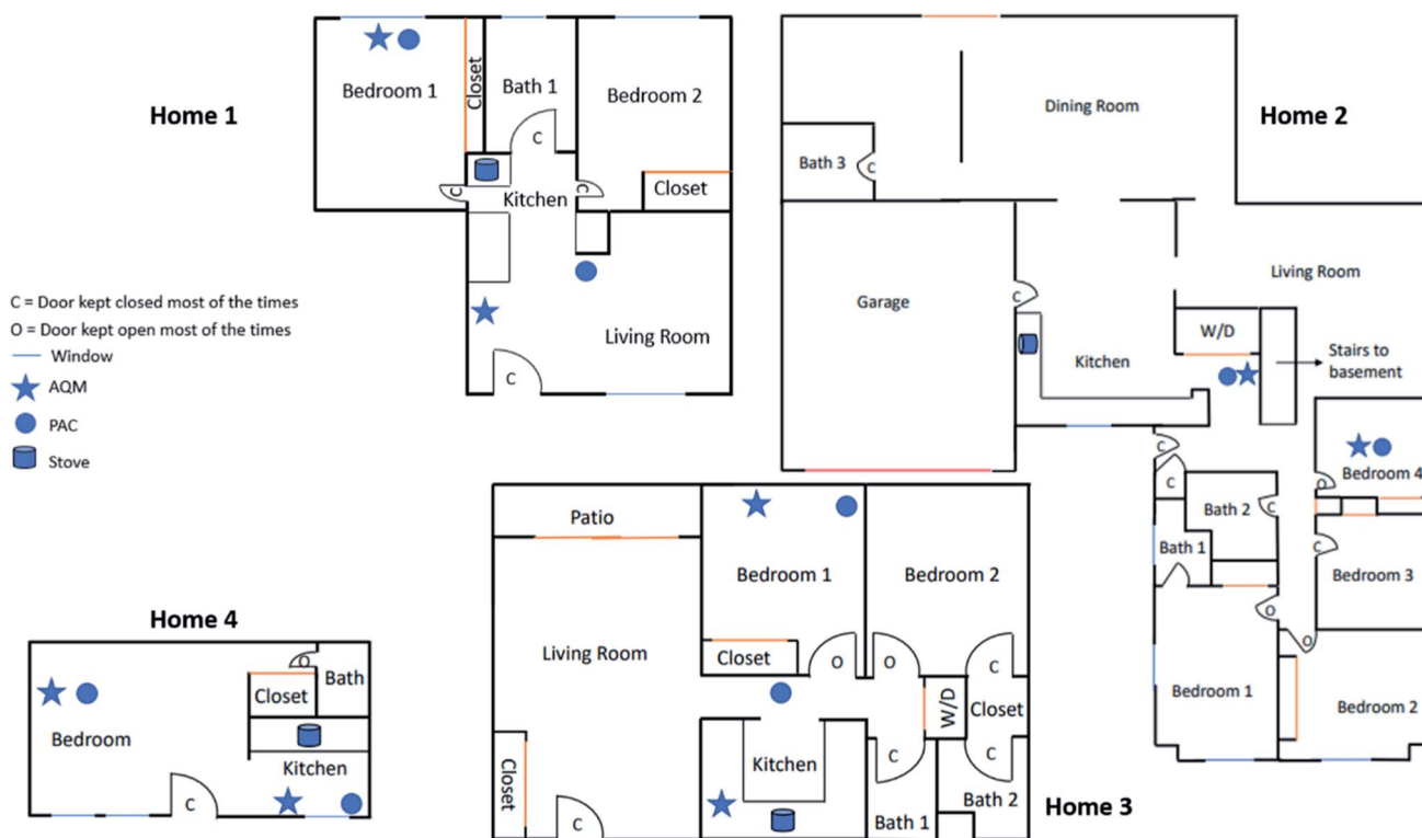
Fig. 1 Layouts for all the locations used for this study. Note all the layouts are approximate to scale (1'':16' for a printed page). The OPS and AQMs were placed on a wire shelf rack, at either 0.3 m or 0.6 m above the floor.
