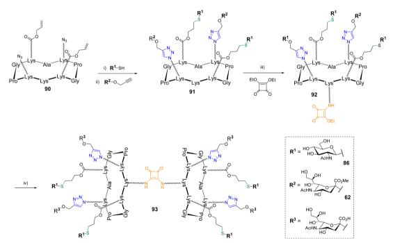
Scheme 18 Synthesis of heterovalent structures using CuAAC, TEC and SqC. Reagents and conditions: (i) DPA, DMF/H<sub>2</sub>O, irrad. 365 nm, r.t., 45 min; (ii) Cu micropowder, PBS (pH 7.4), r.t., 45 min, 71% over two steps; (iii) DMF, DIPEA (pH 8.5), r.t., 4 h, 87%; (iv) 91, Na<sub>2</sub>CO<sub>3</sub> (pH 9.5), 37 °C, 24 h, 67%.
