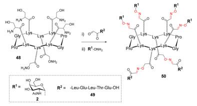
Scheme 10 Functionalization of the second domain of a cyclopeptide scaffold 50 using successive oxime ligation. Reagents and conditions: (i) 0.1% TFA in CH<sub>3</sub>CN/H<sub>2</sub>O (1:1), 37 °C, o/n then NalO<sub>4</sub>, H<sub>2</sub>O, r.t., 1 h, 95%; (ii) 0.1% TFA in CH<sub>3</sub>CN/H<sub>2</sub>O (1:1), 37 °C, o/n, 80%.
