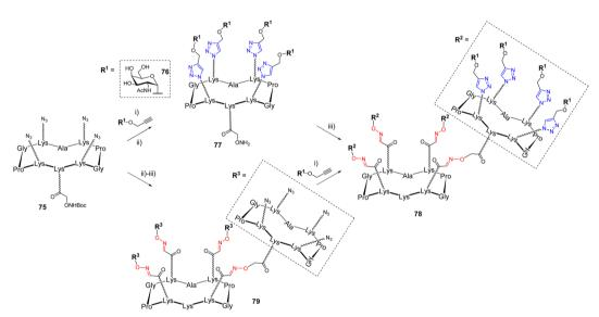
Scheme 15 Convergent synthesis of the hexadecavalent GalNAc glycodendrimer **78** by CuAAC/OL. Reagents and conditions: (i) CuSO<sub>4</sub>·5H<sub>2</sub>O, THPTA, sodium ascorbate, DMF/PBS buffer (pH 7.5) (1:1), r.t., 2 h, 70% (divergent synthesis); (ii) TFA/H<sub>2</sub>O (6:4), r.t., 1 h, 77% over two steps for **77**; (iii) **51**, 0.1% TFA in H<sub>2</sub>O, 37 °C, 45 min, 90% for **78**; 85% for **79**.
