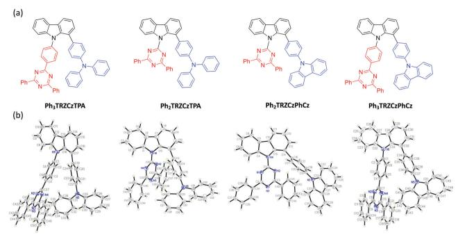
Fig. 1 The chemical structures (a) and X-ray structures (b) of Ph<sub>3</sub>TRZCzTPA, Ph<sub>2</sub>TRZCzTPA, Ph<sub>2</sub>TRZCzPhCz and Ph<sub>3</sub>TRZCzPhCz, thermal ellipsoids were drawn at a 50% probability level.
