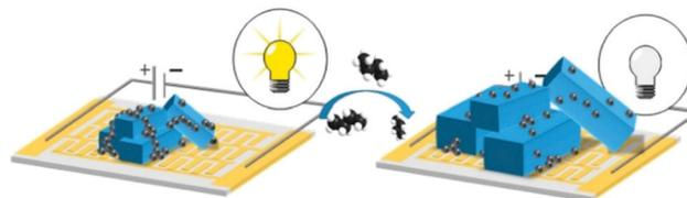
Fig. 5 Switchable MIL-53-carbon additive composite for CO<sub>2</sub> sensing.<sup>25</sup>
