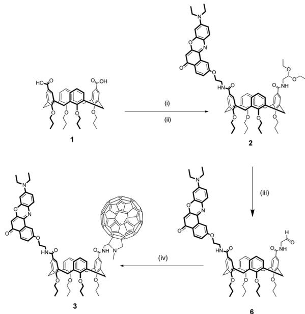
**Scheme 1** Synthesis of Nile Red- $C_{60}$  calix[4]arene **3**: (i)  $(COCl)_2$ , DMF, DCM, 5 h, r.t., quantitative; (ii) 2,2-diethoxyethanamine, **NR-NH<sub>2</sub>**, DIPEA, DCM, 12 h, r.t., 47%; (iii) HCl (1M), dioxane, 4 h, r.t., 77%; (iv)  $C_{60}$ , sarcosine, toluene, reflux, 3 h, 23%.
