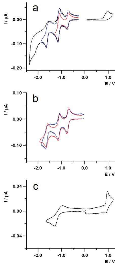
Fig. 4 Cyclic voltammetric curves of (a) 0.6 mM species **3** (three scans at different inversion potential); (b) 0.7 mM compound  $C_{60}$ -Ph (blue line) and **5** (red line); (c) 0.7 mM species **4** recorded in TBAH/DCM at 298 K. Scan rate =  $1 \text{ V s}^{-1}$ ; working electrode: platinum disk (diameter  $125 \mu\text{m}$ ); reference electrode: SCE.
