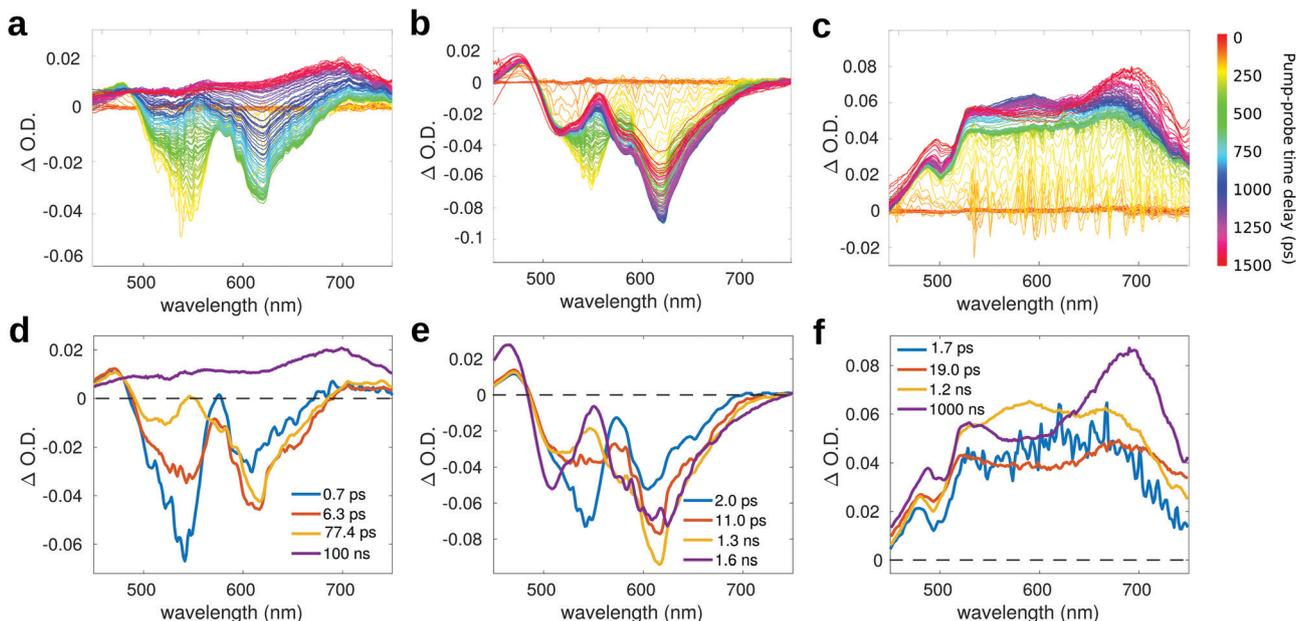
Fig. 6 Transient spectra of: (a) compound **3** ( $\lambda_{\text{exc}} = 530$  nm), (b) compound **4** ( $\lambda_{\text{exc}} = 530$  nm) and (c) compound **5** ( $\lambda_{\text{exc}} = 400$  nm) in toluene. Panels (d–f) report the respective EADS obtained from global analysis.
