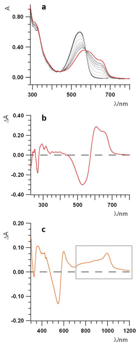
**Fig. 5** (a) UV-Vis-NIR spectra of 0.6 mM dyad **3** in 0.08 M TBAH/DCM solution; working electrode, Pt gauze; temperature = 0 °C. Spectra of the pristine compound (black line) and one-electron reduced species (red line). (b) Difference spectrum of the reduced state (red trace); spectrum of the pristine compound subtracted). (c) UV-Vis-NIR difference spectrum of the oxidized state of dyad **3** 0.6 mM in 0.08 M TBAH/DCM solution; working electrode, Pt gauze; temperature = 0 °C.
