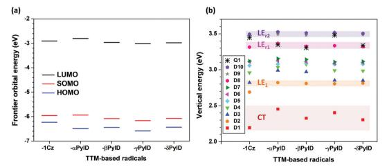
Fig. 2 Energies of (a) the LUMO, SOMO, and HOMO levels and (b) the doublet  $(D_1-D_{10})$  and quartet  $(Q_1)$  states of the TTM-1Cz and TTM-xPyID radicals; CT, LE<sub>1</sub>, LE<sub>1</sub>, and LE<sub>1</sub> represent the D<sub>1</sub>, D<sub>2</sub> (D<sub>3</sub> for TTM-1Cz), D<sub>8</sub>, and D<sub>10</sub> (D<sub>9</sub> for TTM- $\alpha$ PyID) states of the radicals, respectively. All the molecular geometries are the optimized ground-state geometries.
