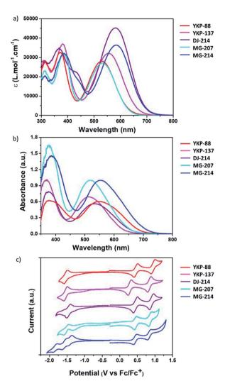
Fig. 3 (a) Absorption spectra registered (a) in Dichloromethane solution, (10 $^{-5}$  M, 25 °C), (b) on 2  $\mu$ m-thick mesoporous TiO<sub>2</sub> electrodes, for compounds YKP-88 (red line), YKP-137 (magenta line), DJ-214 (violet line) MG-207 (cyan line) and MG-214 (blue line) (c) cyclic voltammetry traces in solution for each compound (deoxygenated dichloromethane,  $10^{-3}$  M, 25 °C, voltage scan 200 mV s<sup>-1</sup>).
