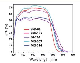
Fig. 4 External Quantum Efficiency (EQE) spectra of solar cells fabricated with YKP-88, YKP-137, DJ-214, MG-207 and MG-214.
