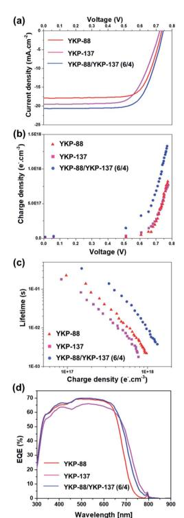
Fig. 5 (a) Current-voltage (J, V) curves for YKP-88, YKP-137 and YKP-88/YKP-137 (6/4) devices, (b) charge extraction data showing electron density as a function of induced voltage for the corresponding DSSCs (c) transient photovoltage data showing electron lifetimes versus electron density. (d) Comparison of the IPCE spectra of YKP-88-, YKP-137-based solar cells and the co-sensitized device (ratio 6/4).
