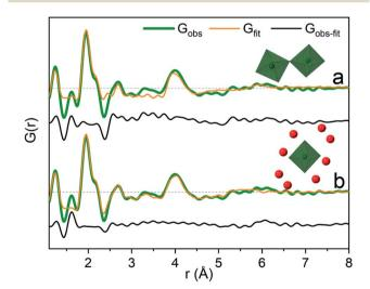
Fig. 3 PDF of the 1 M solution of  $Ga(NO_3)_3$  with R=0 modelled with (a) octahedrally coordinated  $Ga^{3+}$  in a dimer ( $R_w=0.412$ ) and (b) a monomer with a second solvent shell ( $R_w=0.284$ ). The two models are shown as insets with green ochatedra representing  $GaO_6$  and solvent oxygen as red spheres.
