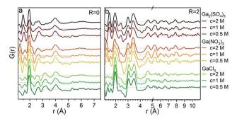
Fig. 11 PDF data for aqueous solutions of  $Ga(NO_3)_3$ ,  $GaCl_3$ , and  $Ga_2(SO_4)_3$  with concentrations of 0.5, 1 and 2 M. (a) R=0 and (b) R=2. The variations between the salts is due to differences in pH as outlined in Fig. 1b and Table S12.†
