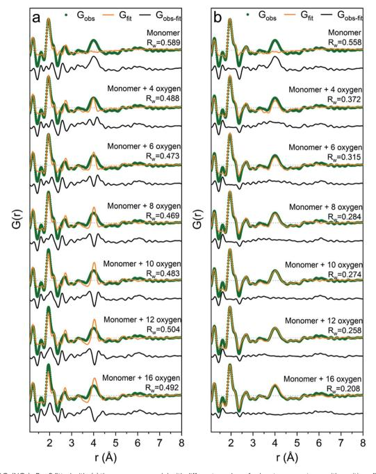
Fig. 5 PDFs of  $Ga(NO_3)_3$  R=0 fitted with: (a) the monomer model with different number of solvent oxygen atoms with positions fixed at values in a crystal structure<sup>37</sup> and (b) the same models with refined oxygen positions and a box restraint of  $\pm 0.2$  Å.
