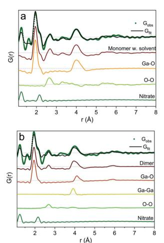
Fig. 4 Model calculation of partial PDF contribution to (a) the monomer with the solvent and (b) the dimer model.
