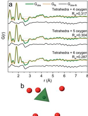
Fig. 9 (a) PDFs of the  $Ga(NO_3)_3$  solution with R=4 modelled with tetrahedrally coordinated  $Ga^{3+}$  including anions 4, 5 and 6 solvent oxygen atoms. (b) The refined structure with 5 solvent oxygen atoms is shown as the inset with the green tetrahedra representing  $GaO_4$  and oxygen as red spheres.
