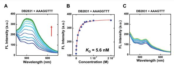
Fig. 3 Fluorescence emission spectra for 10 nM DB2831 titrated with sequence AAAGGTTT (A), or AAAGTTT (C) in TNE100 buffer at 25 °C. The excitation wavelength is 390 nm, respectively. The slit widths are [20, 20 nm]; fluorescence binding curve between 10 nM DB2831 and tested sequences in TNE100 buffer to determine equilibrium constant. Full DNA sequences as described in Fig. 1C.
