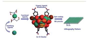
Scheme 1 Illustration of the assembly of the atomically precise In<sub>12</sub>-oxo clusters with chemical modification and patterning evaluation.
