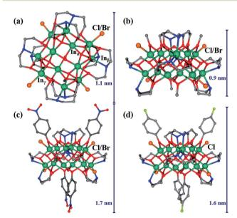
Fig. 1 (a) Molecular structure of InOC-1 and InOC-2 in top views. (b) Molecular structure of InOC-1 and InOC-2 in side views. (c) Molecular structure of InOC-3 and InOC-4 in side views. (d) Molecular structure of InOC-5 in side views. Atom color code: dark-green, In; red, O; blue, N; gray, C; orange, Cl or Br; lime, F. All H atoms have been omitted for clarity.
