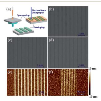
Fig. 4 (a) Schematic illustration of the patterning process of  $In_{12}$ -oxo clusters. SEM images of patterns with 200 nm lines obtained using electron-beam lithography performed with a dose of 1000  $\mu$ C cm<sup>-2</sup> for InOC-1 (b), InOC-2 (c) and InOC-3 (d). AFM images of patterns obtained with a dose of 500  $\mu$ C cm<sup>-2</sup> exhibiting feature sizes of 200 nm (e) and 50 nm (f) for InOC-3.
