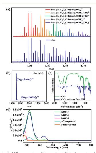
Fig. 3 (a) The comparison of the experimental isotopic envelope with simulated patterns of the predominant species of  $\{\ln_{12}\text{-cluster}\}^{2+}$  and (b) positive-mode ESI-MS entire spectrum of InOC-1 in DMF; (c) comparison of the FT-IR spectra of InOC-1 (olive) and InOC-1 dissolved in DMF followed by extraction with the assistance of PGMEA (navy); (d) comparative UV-Vis spectra of InOC-3, InOC-4, InOC-5 and their corresponding free ligands p-nitrophenol and p-flurophenol in DMF.
