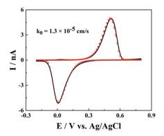
Fig. 6 The cyclic voltammograms of 1 mM FeCl<sub>3</sub> in 0.5 M H<sub>2</sub>SO<sub>4</sub> and 0.1 M KCl from the simulation (red points) and experiments (black solid line). a = 100 nm. d = 1320a, tan  $\theta = 0.2$ , v = 0.1 V s<sup>-1</sup>,  $E_0 = 0.26$  V and  $k_0 = 1.3 \times 10^{-5} \text{ cm s}^{-1}$ .
