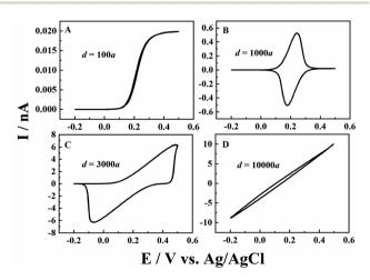
Fig. 3 Simulated i-V responses from a CNP at different solution depths in 1 mM  $K_4Fe(CN)_6 + 0.1$  M KCl. From panels (A) to (D), the solution depth is 100a, 1000a, 3000a, and 10 000a. a = 50 nm, tan  $\theta =$ 0.2.  $v = 0.1 \text{ V s}^{-1}$  and  $E^0 = 0.2 \text{ V}$ .
