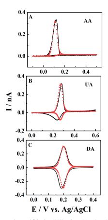
Fig. 7 The experimental (black solid lines) and simulated (red points) voltammograms of AA, UA and DA in CNPs. The concentration is 0.5 mM with 10 mM PBS (pH 7.4) buffer. Fitted value: a = 50 nm, d = 0.5800a, tan  $\theta = 0.15$ , and  $v = 0.1 \text{ V s}^{-1}$ .  $k_c > 0.8$ ,  $k_c = 0.2$ , and  $k_c < 0.01 \text{ s}^{-1}$ and  $E_0 = 0.11/0.27/0.2 \text{ V}$  for AA, UA and DA.
