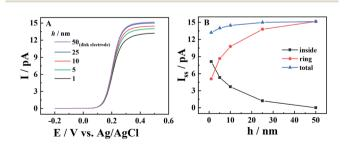
Fig. 1 The simulated steady-state voltammograms of CNPs with different thicknesses (h) of deposited carbon. The solution is 1 mM  $K_4$ Fe(CN)<sub>6</sub> + 0.1 M KCl. a=(50-h) nm, d=400a,  $\tan\theta=0.2$ , v=0.1 V s<sup>-1</sup> and  $E^0=0.2$  V vs. Ag/AgCl.
