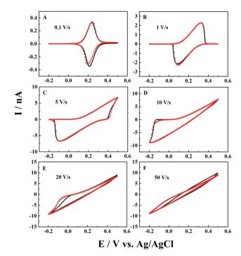
Fig. 2 Effect of scan rate on i-V curves in 1 mM K<sub>4</sub>Fe(CN)<sub>6</sub> + 0.1 M KCl. From panels (A) to (F), the experimental (black solid lines) and simulated (red points) i-V curves are at scan rates of 0.1, 1, 5, 10, 20, and 50 V s<sup>-1</sup>. Fitting parameters: a=50 nm, d=2000a,  $\tan\theta=0.2$  and  $E^0=0.21$  V.
