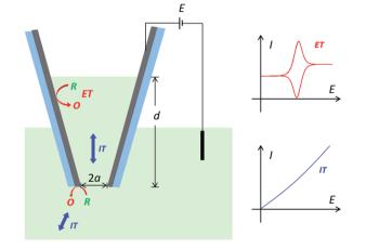
Scheme 1 The charge transport processes in carbon nanopipettes. When applying a potential at the carbon layer, the measured current signal would be determined by both the ion transport processes in the nanopipette and the electron transfer processes at the carbon layer.
