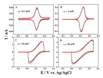
Fig. 4 Experimental (black solid lines) and simulated (red points) i-Vcurves for different concentrations of K<sub>4</sub>Fe(CN)<sub>6</sub> (c<sub>0</sub>). The background solution is 0.1 M KCl. a=50 nm, d=1000a,  $\tan\theta=0.2$ , v=0.1 V s<sup>-1</sup> and  $E_0 = 0.21 \text{ V}$ , 0.24 V, 0.2 V, and 0.25 V.
