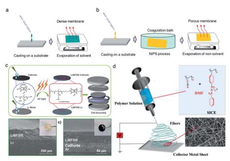
Fig. 9 Schematic illustration of membrane fabrication methods. (a) Casting method. (b) NIPS phrase separation. (c) *In situ* polymerization. Reproduced with permission.<sup>94</sup> Copyright 2020, American Chemical Society. (d) Electrospinning technique. Reproduced with permission.<sup>96</sup> Copyright 2017 Wiley.
