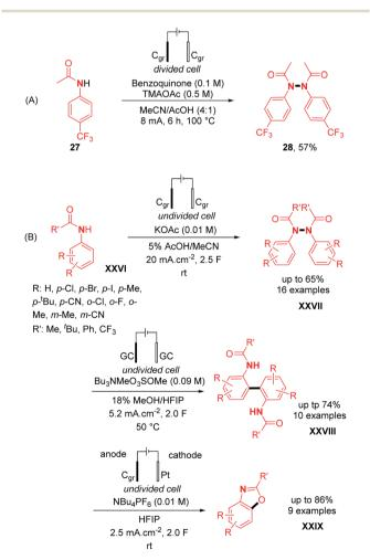
Scheme 14 Dehydrogenative anodic oxidation of anilides for N-N bond formation.
