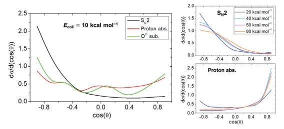
Fig. 4 Normalized scattering angle distributions of the  $OH^- + CH_3F$  reaction are presented for  $S_N2$  ( $F^- + CH_3OH$ ), proton abstraction ( $H_2O + CH_2F^-$ ) and oxide anion substitution ( $HF + CH_3O^-$ ) at a collision energy of 10 kcal mol<sup>-1</sup>. The angular distributions of  $S_N2$  and proton abstraction are also shown at collision energies of 20, 40, 50 and 80 kcal mol<sup>-1</sup>.
