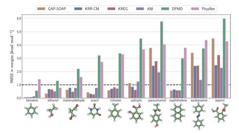
Fig. 3 Performance of MLPs trained only on energies. Root-mean squared error (RMSE) calculated for energies with different ML potentials for all molecules of the MD17 database. The models were trained on a sub-sample of 1000 molecular geometries for each system. The reported RMSE values correspond to the average of the test errors for 20 independently trained models evaluated on a test set with 20k geometries.
