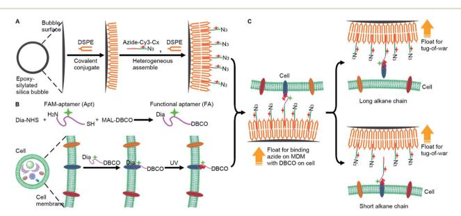
Fig. 1 Schematic illustration of the molecular dynamometer (MDM), functional aptamer (FA), and "tug-of-war" tests. (A) Preparation of the MDM. (B) Preparation and conjugation of the FA with the target protein on the cell membrane. (C) Binding of the MDM with the FA-conjugated cells for "tug-of-war" tests.
