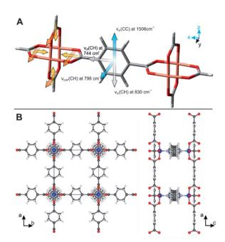
Fig. 7 (A) Illustration of the transition dipole moments for the aromatic vibrations found in the BDC linker. (B) Crystal structure of  $Cu_2(-BDC)_2DABCO$  with the proposed aromatic linker orientation perpendicular to the carboxylate plane.
