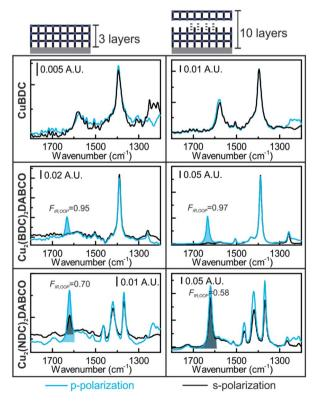
Fig. 6 Polarization-dependent ATR-IR spectra of MOF films prepared with the layer-by-layer method with 3 and 10 layers. The  $\nu_{\rm asymm}(-COO^-)$  band of both 3D MOFs, Cu<sub>2</sub>(BDC)<sub>2</sub>DABCO and Cu<sub>2</sub>(1,4-NDC)<sub>2</sub>DABCO, shows strong polarization dependence, which allows to calculate the degree of out-of-plane orientation from the band areas. Background = blank Si ATR crystal.
