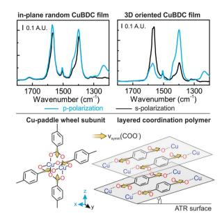
Fig. 8 (Top) Polarization-dependent ATR spectra of CuBDC prepared from random and aligned Cu(OH)<sub>2</sub>. Background spectrum = blank Si ATR crystal. (Bottom) Cu-paddle wheel subunit found in 2D MOFs and BDC linker alignment in a layered coordination polymer. The transition dipole moment of the  $v_{\rm symm}({\rm COO}^-)$  bands are indicated by yellow arrows.
