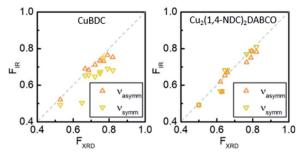
Fig. 3 Correlation of degree of orientation F obtained from XRD and FTIR spectroscopy in transmission for CuBDC and Cu<sub>2</sub>(1,4-NDC)<sub>2</sub>-DABCO films for  $v_{\text{symm}}(\text{COO}^-)$  and  $v_{\text{asymm}}(\text{COO}^-)$  bands.
