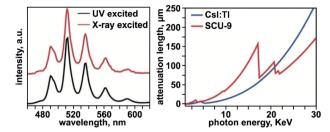
Fig. 6 (Left) Emission profile of  $UO_2(HBTA)(H_2O)$  (SCU-9) under UV (black) and X-ray (red) excitation. (Right) X-ray attenuation lengths for  $UO_2(HBTA)(H_2O)$  (red) and CsI:Tl (dark blue) in the X-ray energy region ranging from 30 eV to 30 keV. Reproduced from ref. 224 with permission from John Wiley and Sons, Copyright 2018.
