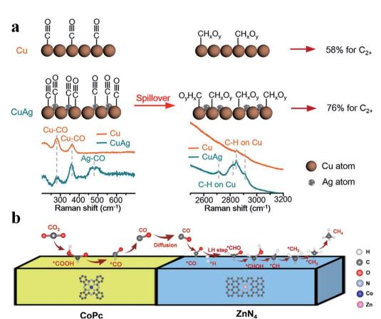
Fig. 12 (a)  $CO_2RR$  mechanism for producing  $C_{2+}$  products on Cu and CuAg catalysts. Reproduced with permission from ref. 113. Copyright (2019) American Chemical Society. (b) A proposed reaction mechanism of the  $CO_2RR$  to  $CH_4$  over COPc@Zn-N-C. Reproduced with permission from ref. 116. Copyright (2020) Wiley-VCH.
