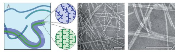
Fig. 2 (A) Schematic diagram of fibre-like  $PMeOx_m$ -b- $PiPrOx_n$  nanorods showing crystalline PiPrOx core with a rectangular cross-section (green) and a solvated PMeOx corona (blue). (B) TEM image of  $PMeOx_{48}$ -b- $PiPrOx_{47}$  nanorods prepared by annealing a 2 mg mL<sup>-1</sup> aqueous solution at 70 °C for 1 week. (C) Magnification of area outlined in (B). Scale bars equal to 200 nm.
