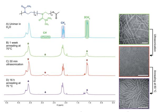
Fig. 3 Concomitant nanofibre fragmentation and BCP dissolution. Left,  $^1$ H NMR spectra (400 MHz, 2 mg mL $^{-1}$  in D $_2$ O) of PMeOx $_{48}$ -b-PiPrOx $_{47}$  unimer (A), nanofibres prepared annealing the BCP solution at 70 °C for 1 week (B), a mixture of seed fragments and BCP unimer prepared via ultrasonication (C) and elongated seeds (D). Right, TEM images showing polydisperse nanofibres (top), seeds (middle) and elongated seeds (bottom). Scale bars equal to 250 nm.
