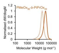
Fig. 1 SEC chromatograms (RI, DMAc 0.03 wt% LiBr,  $1 \text{ mL min}^{-1}$ ) of PMeOx<sub>m</sub>-b-PiPrOx<sub>n</sub> block copolymers (solid line) and PMeOx<sub>m</sub> homopolymers (dashed line) characterised prior to iPrOx addition.
