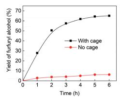
Fig. 4 Yields of furfuryl alcohol *vs.* time in the presence of 9 mol% cage (black line and squares) or in the absence of cage (red line and circles). Yields in the presence of cage are isolated yields. Yields in the absence of cage were determined by <sup>1</sup>H NMR and are likely to be slight overestimates of the amount of furfuryl alcohol produced.
