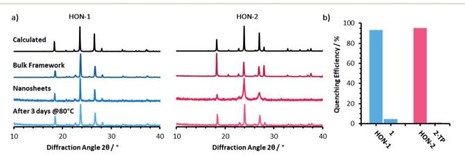
Fig. 4 (a) Powder X-ray diffractometry patterns for both the one (blue) and two (pink) component systems, of: the calculated and as synthesised frameworks, nanosheets, and water treated nanosheets. (b) The quenching efficiencies of hydrogen-bonded framework nanosheets and bulk frameworks towards Rhodamine B fluorescence ( $\lambda_{\rm ex} = 556$ ,  $\lambda_{\rm em} = 577$  nm). Emission titration spectra can be seen in Fig. S21–S24.†
