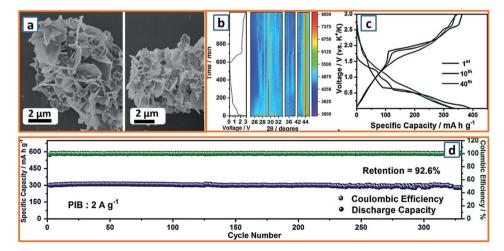
Fig. 16 Potassium storage chemistry and applications of conversion—decomposition-type anodes. (a) Morphology of crystal-pillar-like CuSe. (b) *In situ* XRD patterns of the CuSe electrode obtained during the first electrochemical cycle. (c) Charge—discharge curves and (d) long cycling performance of CuSe electrodes in KIB. Reproduced with permission.<sup>20</sup> Copyright 2019, Wiley.
