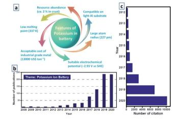
Fig. 1 (a) Various features of potassium in batteries. (b) Literature distribution of KIB based research from 2008 to 2020 in the website of Web of Science, and (c) corresponding number of citations.
