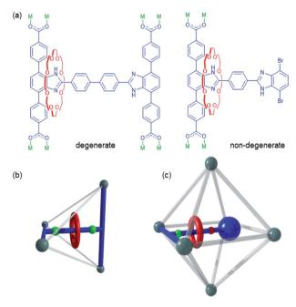
Fig. 1 (a) The degenerate molecular shuttle (left) previously incorporated into the Zr(v) MOF UWDM-8 and the non-degenerate molecular shuttle (right) incorporated into UWDM-11; this work. (b) A schematic representation of the tetrahedral cavity of UWDM-8 crosslinked with a degenerate molecular shuttle. (c) The octahedral cavity of UWDM-11 featuring a non-degenerate molecular shuttle appended to one of the linkers.
