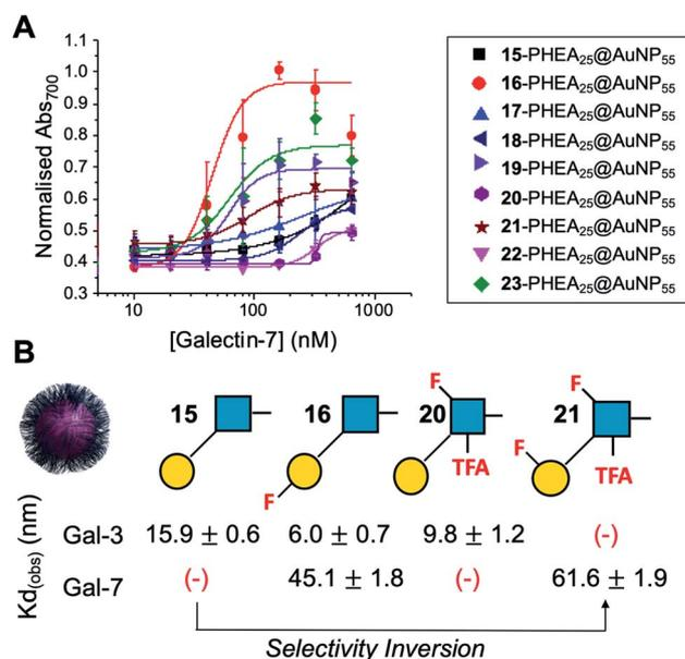
Fig. 5 Galectin-7 binding to the F-glyconanoparticle library. (A) Dose-response curve for the AuNP aggregation assay; (B) summary of apparent  $K_D$  (nM) for selected glycans showing the fine-tuning and selectivity inversion. (-) = no binding.
